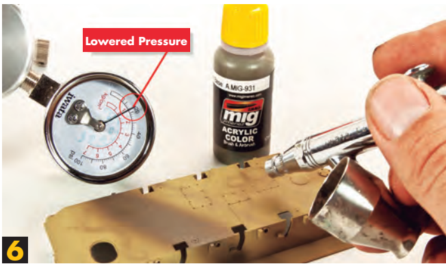
6 Now with the primer in place and the pressure lowered it is time to paint. I am using an Iwata Dual Action Airbrush; note the distance of the airbrush nozzle to the surface is approximately 3" inches for an overall spray. I will move my nozzle closer to the surface when applying fine lines and details. As with the primer, I will work layer by layer to achieve full coverage.
